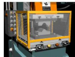
Fixed Barrier Guard on a Power Press
